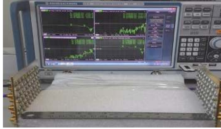
FIGURE 8: Measurement setup established by connecting one patch to two arrays, placing two arrays face-to-face at a distance of R = 19.5 cm, and testing the 2-port S-parameters using the Rohde & Schwarz ZVA40 vector network analyzer.
