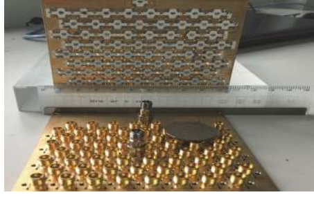
FIGURE 7: Photograph of two identical mmW microstrip arrays for testing.
