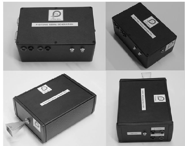
Fig. 15 Photographs of the developed subsystems. (a) and (b) show the photonic mm-wave unit, (c) the wireless 60 GHz transmitter and (d) the wireless receiver.
