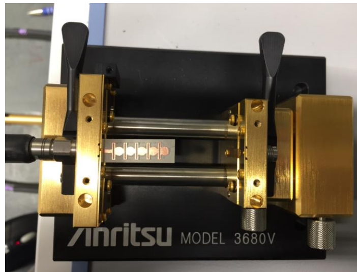
Figure 37 Antenna measured with Anritsu 3680V test fixture
