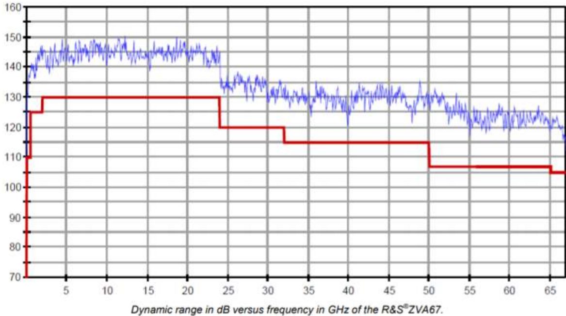
Figure 39 R&S ZVA67 vector network analyzer dynamic range [69]
