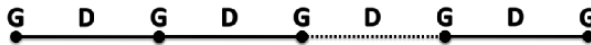
Figure 2 – Positions where the one dimensional Gradient (G) and Divergence (D) are calculated.
