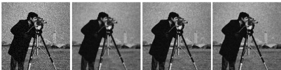
Figure 7 – (Left to Right) Noisy image of the Cameraman perturbed by Gaussian additive noise of zero mean and variance \nu = 0.01 . Filtered image of the Cameraman after 17 iterations by the finite difference method. Filtered image of the Cameraman after 4 iterations by the finite element method. Filtered image of the Cameraman after 6 iterations by the mimetic discretization method.
