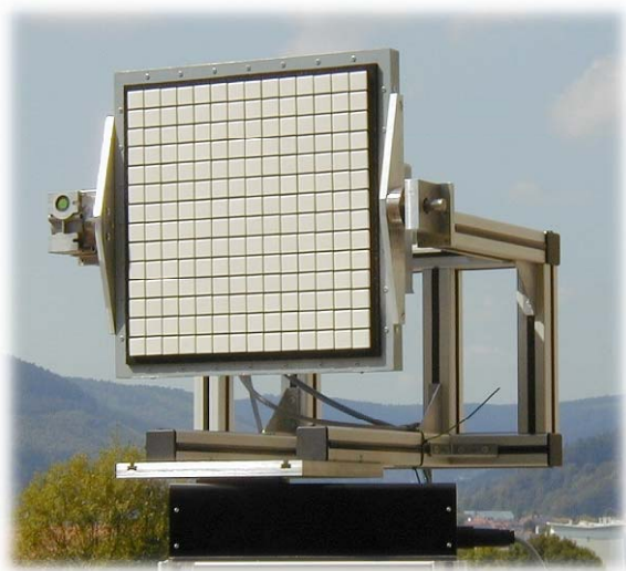
Figure 4: 8x8 URA designed for 5.2 GHz.
