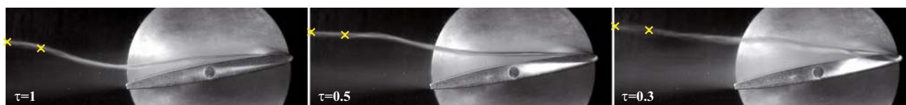
Fig. 6 Superposition of the cavitating TLV visualizations during 11 ms for three gap widths. The yellow crosses represent the position measured by SPIV in cavitation-free regime, in the planes z/c = 1 and 1.2. Flow conditions: W_\infty = 10 m/s, incidence = 10°, p_\infty = 1 bar
