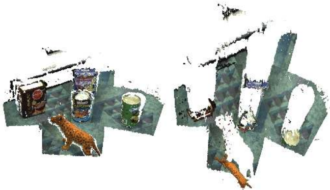
Fig. 1. Example for a point cloud representing a whole scene merged from different view points. Left: View from the side. Right: View from the top.
