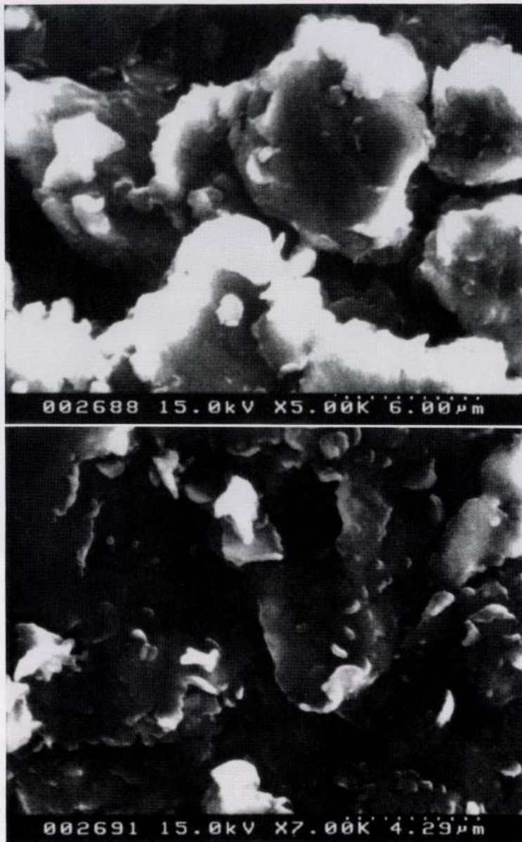
FIG. 11. Scanning electron micrographs (SEM) of the mixed-layer kaolinite/smectite minerals in a fine sample from C layer. Both photographs reveal stacked flakes of the interstratified minerals with faint irregular outlines and curled edges.
