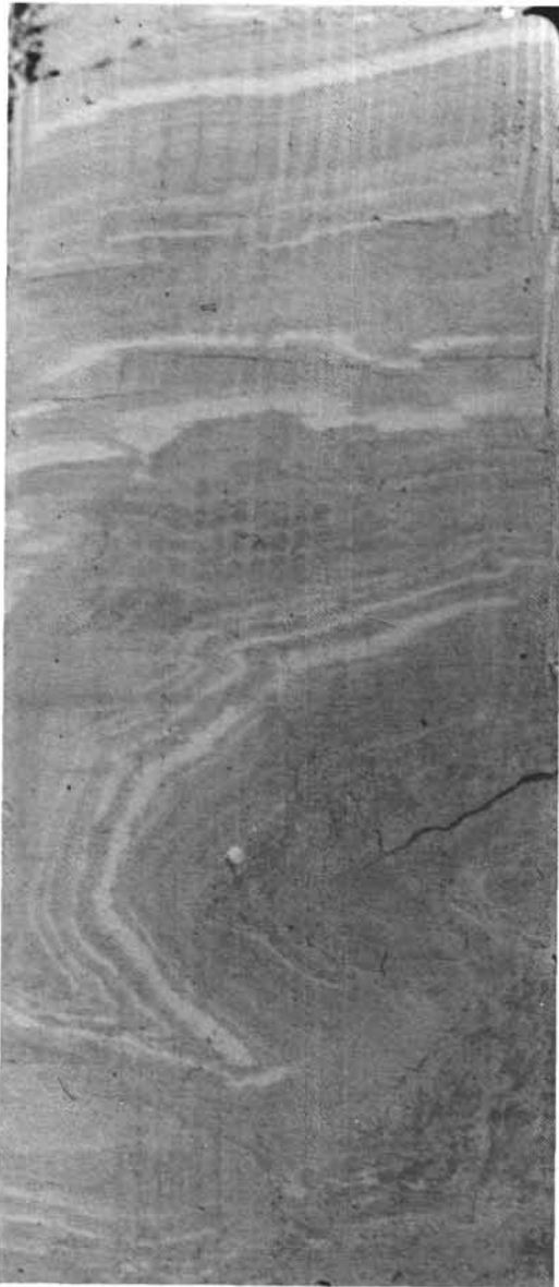
Figure 7. Laminated anhydrite. The rock consists of massive anhydrite displaying original bedding. This bedding was displaced by the growth of white nodules of anhydrite at the time the sediment was still soft (124, core 8, on scale).
