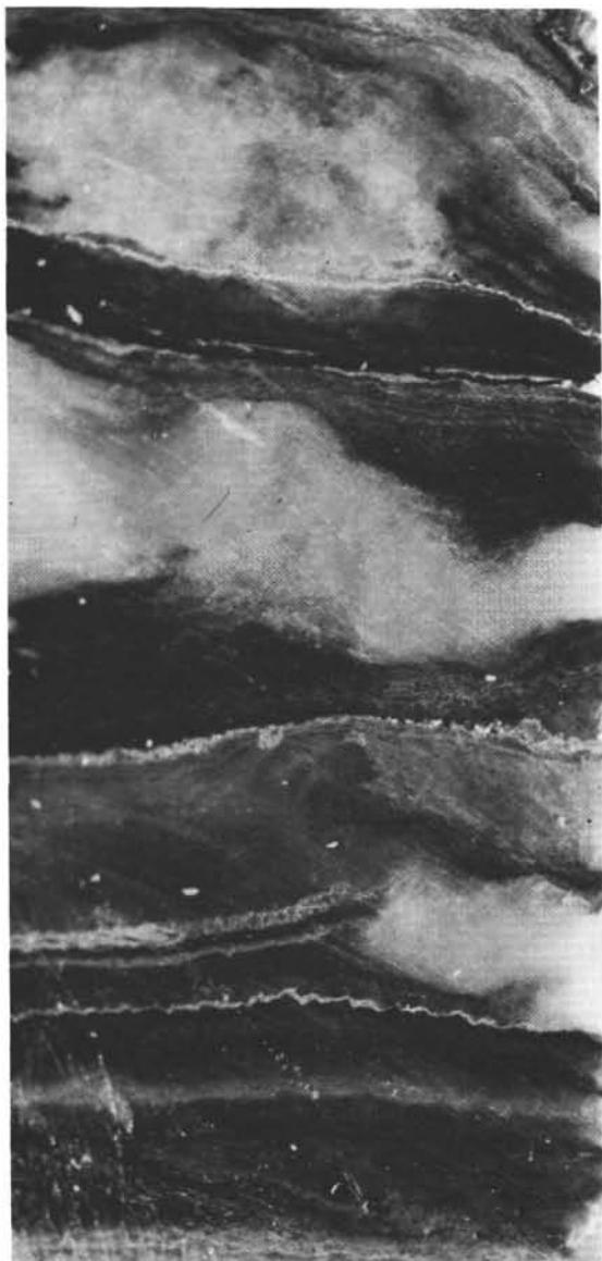
Figure 14. Massive gypsum. Black and white beds separated by thin wavy boundaries. Tyrrhenian Sea (132-27-1, 50-80 cm, on scale).
