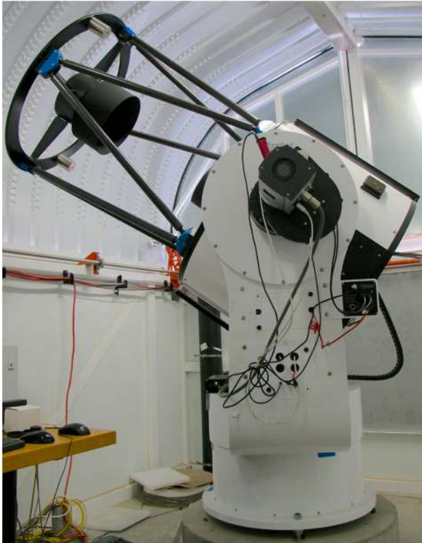
Fig. 3 Telescope 2, a PlaneWave CDK-700, is shown inside the MINERVA Aqawan telescope enclosure at the Caltech commissioning site.
