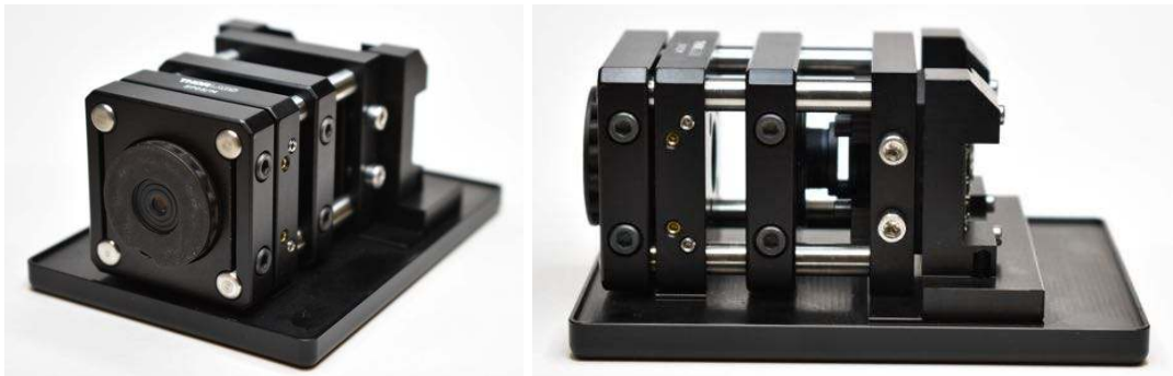
Figure 3: Interchangeable optomechanics mounted to baseplate.
