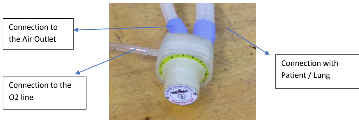
Figure 1. Reverse Engineering of the prototyped Takaoka 600 Mini-Respirator per 3D Printer.
