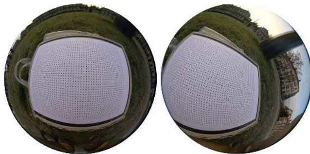
Figure 6. Two images of the grids used for calibrating the fisheye lens.
