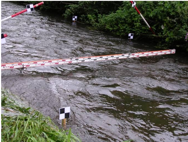
Figure 3. Survey staff positioned close to the water surface
