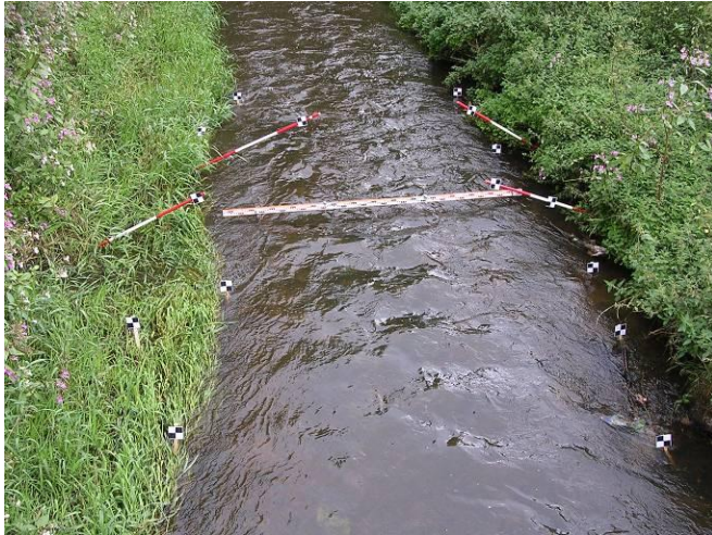
Figure 2. Target point setup on the river in Loughborough
