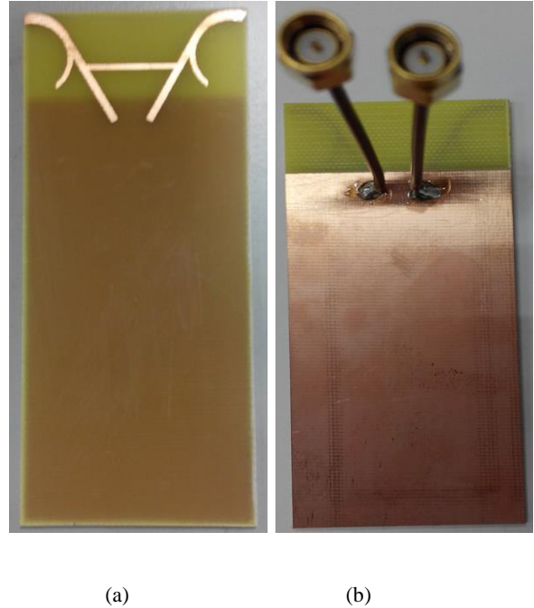
Figure 5. Practical prototype of the proposed antenna (a) top view (b) back view.
