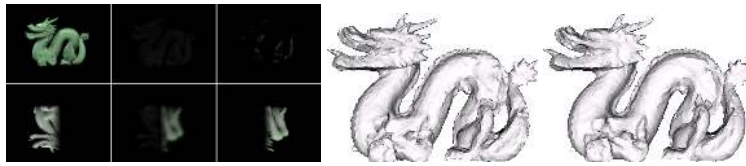
Figure 5: Dragon sequence synthesized with specular reflectance model and occlusions. From left to right : 2 of 32 input images; recovered corrective images; ground truth corrective images; recovered shape without the corrective model; recovered shape with the corrective model.
