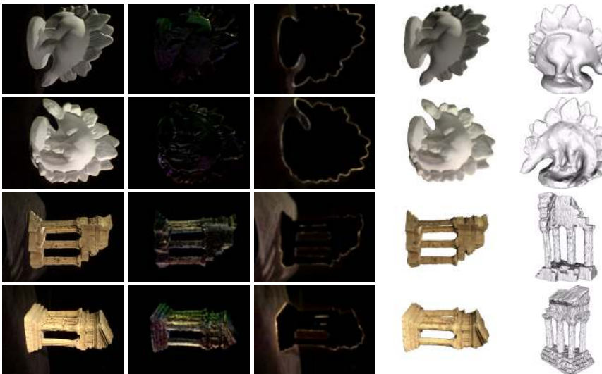
Figure 6: Dino and Temple sequence. From left to right: 1 of 16 input images; estimated non-Lambertian component (scaled by 8 for visualization); estimated background images (scaled by 2 for visualization); estimated radiance; estimated mesh seen from a different viewpoint.
