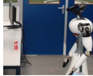
Fig. 7. The AMIGO robot must driver closer to the table to be able to grasp the red can.
