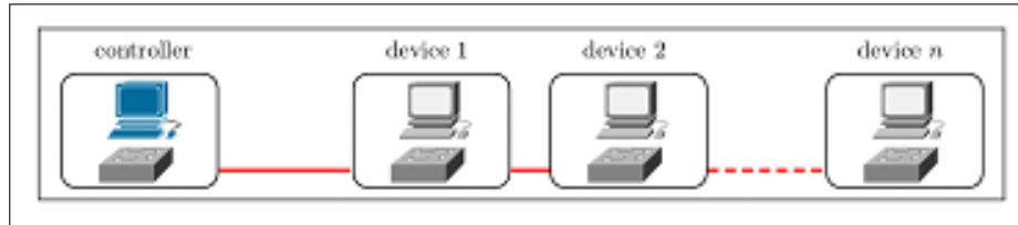
Figure 5: Profinet line topology
