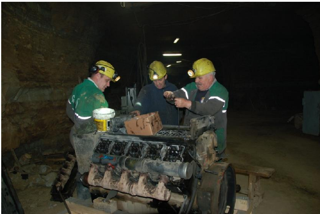
Illustration 7. Mechanics repairing an engine in the underground garage
