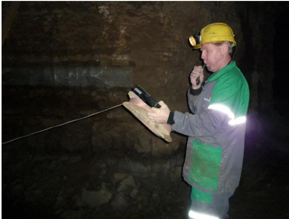
Illustration 8. A blaster whistling as a warning for everyone to leave the area before he sets off the blast from his detonator
