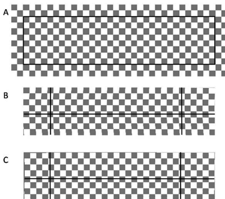
Fig. 1. Checkerboard patterns created in software (Matlab function ‘checkerboard’). The initial checkerboard is shown in (A). Two projective transformations were created based on experimental data using the RXN-1 spectrograph, for the forward transform (a corrective transform) and the inverse transform (a transform introducing distortions to the image). The initial checkerboard was transformed with the inverse transform to simulate an image recorded through the spectrograph optics, as shown in (B). Straight reference lines (black) have been inserted to improve visualization of curvature and rotational misalignment in the image. The rotational misalignment is very slight, approximately -2 vertical pixels over 1024 pixels, or -0.1 degrees. The imperfect image of (B) was then forward transformed to obtain a corrected image, shown in (C).
