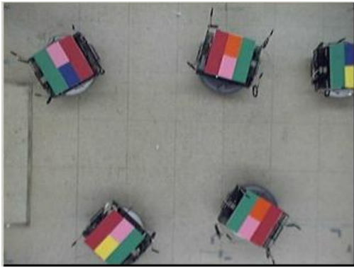
Figure 7: The webcam shot of the testbed. The color patch on each node uniquely identifies the node as well as tells its position and orientation.
