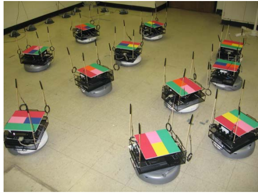
Figure 1: MiNT-m prototype with 12 mobile nodes and charging stations (top left corner of the image).
