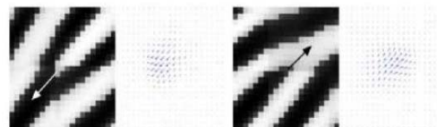
Fig. 16 Symmetry filter response in the minutia point. Left-ridge bifurcation, Right-ridge ending.
