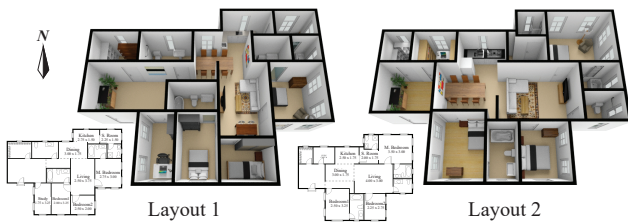
Figure 9: Two apartment layouts are generated by our algorithm with the same input. Boundary constraints are added for bedrooms to ensure that all bedrooms receive sufficient sunshine from the south east direction. The north direction is shown.
