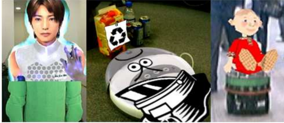
Figure 10: MiRAs with Mixed Reality embodiment. From left to right: U-Tsu-Shi-O-Mi (Virtual Humanoid), Jeeves, and Dragone et al.'s MiRA.
