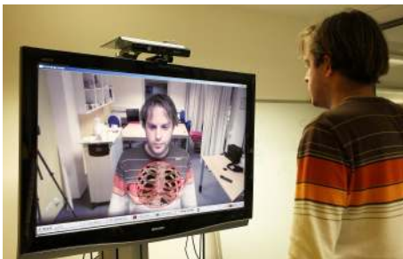
Figure 1: The system consists of a display device, a color camera and a depth camera. The user is tracked and a CT dataset is augmented onto the user.
