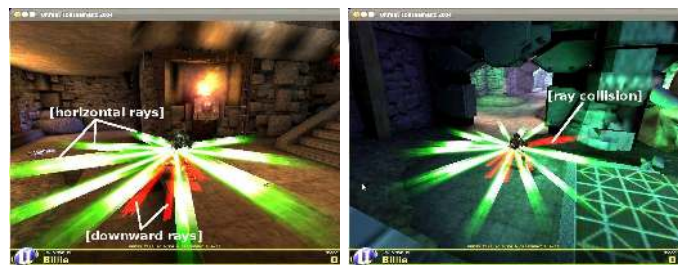
Fig. 4. Backup navigation based on ray casting
