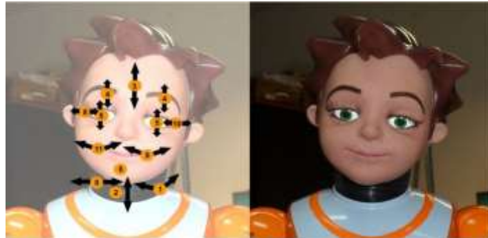
Figure 4.2.3-1 Mapping of the servo motors on the face and the neck of ZECA (Costa, 2014).
