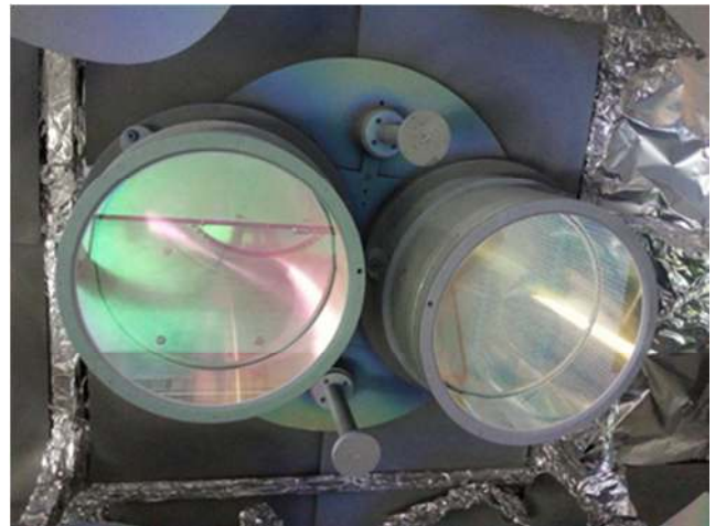
Fig. 10: Two Ø35 cm IM installed in the coater sample holder
