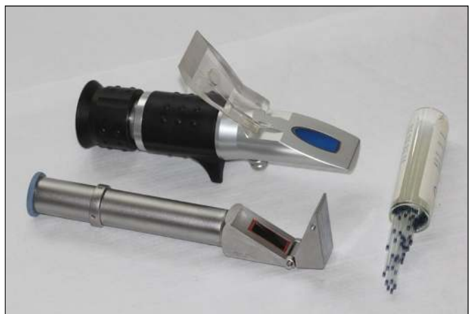
Fig. 35. Calibrated micropipettes/ micro-capillary tubes and refractometers used for measurements of nectar concentration and volume. Photo: A Switala.
