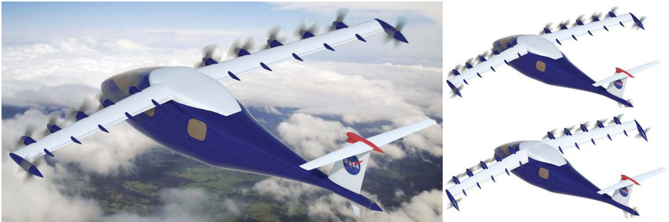
Figure 7: NASA Langley LEAPTech Distributed Electric Propulsion concept, that coupled highly integrated propulsion and control with a variable wing incidence highlift system (images on right are at the takeoff 19 degree and landing 34 degree conditions), high aspect ratio wing, and fuselage boundary layer ingestion propulsion.
