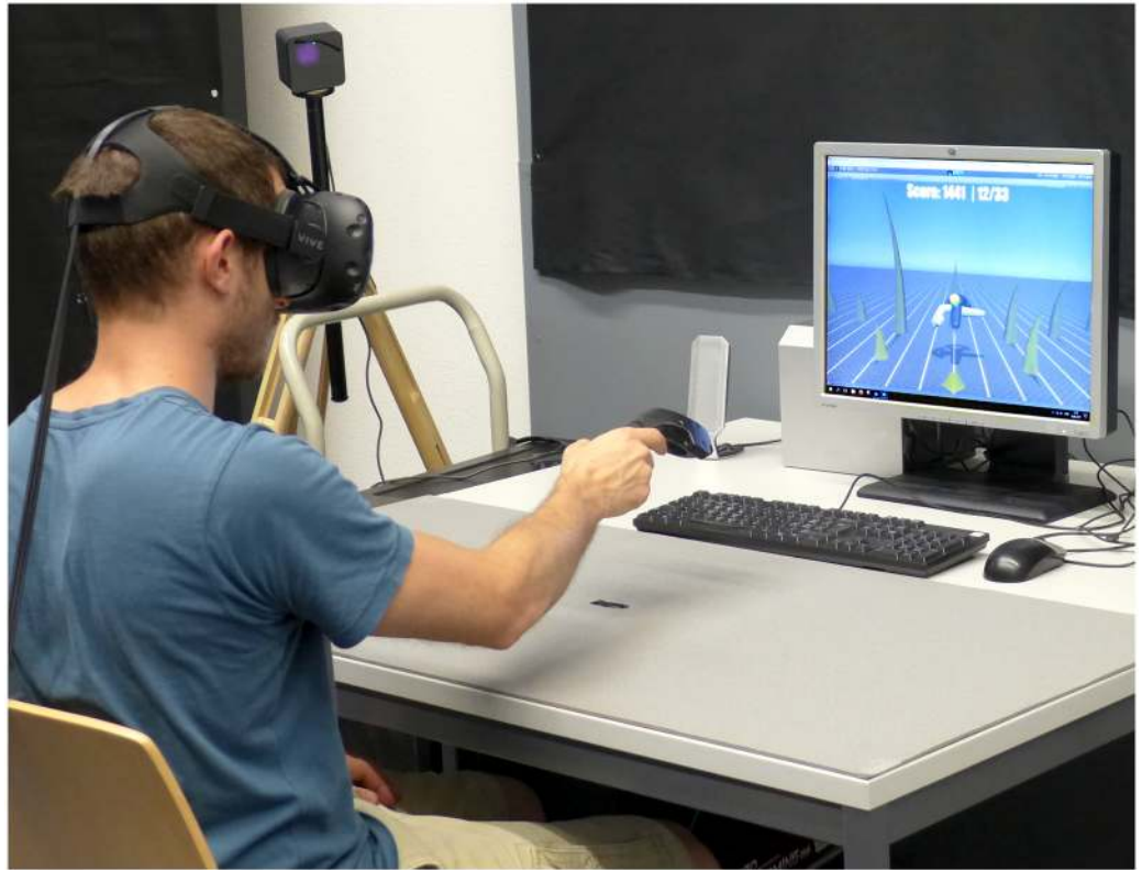
Fig 1. Subject using the experimental setup. The subject sat at the cushioned table with resting position indicated with a stripe in the table center. Handheld (right hand) and head-mounted display (head) were tracked by the Lighthouse with one base station visible in the back. The desktop monitor was located and oriented as used during experiments without the head-mounted display. A clearer picture of the virtual scene with better contrast and colors is provided in Fig 2. The depicted individual is the corresponding first author. The individual in this manuscript has given written informed consent (as outlined in PLOS consent form) to publish these case details.
