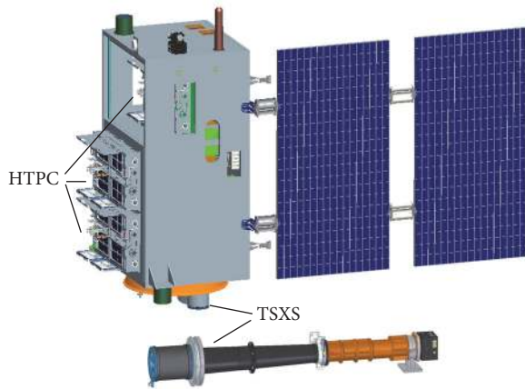
FIGURE 2: XPNV-1 satellite structure overview.
