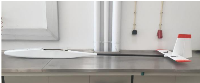
Figure 3 - Improved LEEUAV fuselage, tail boom and tail control surfaces made by Duarte [6]
