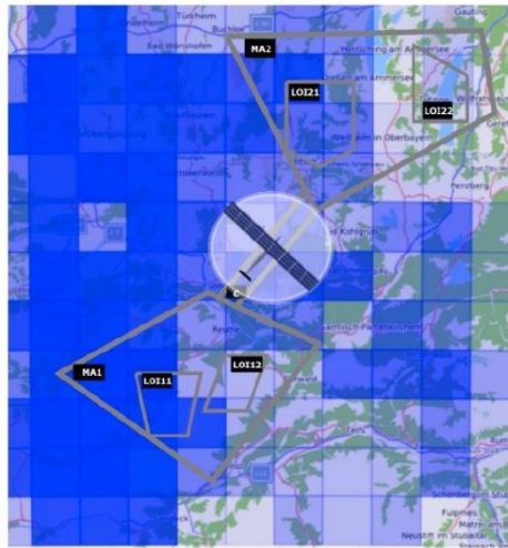
Figure 17 - Cloud coverage map containing mission areas (MA) and locations of interest (LOI) where the UAV will perform surveillance within a time frame, in the MMS application test [42]
