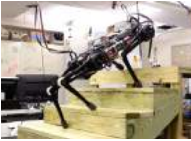
Fig. 7: Blindly Climbing Stairs. With the control framework described throughout the paper, the robot was able to successfully climb up stairs without the use of external environment sensors.
