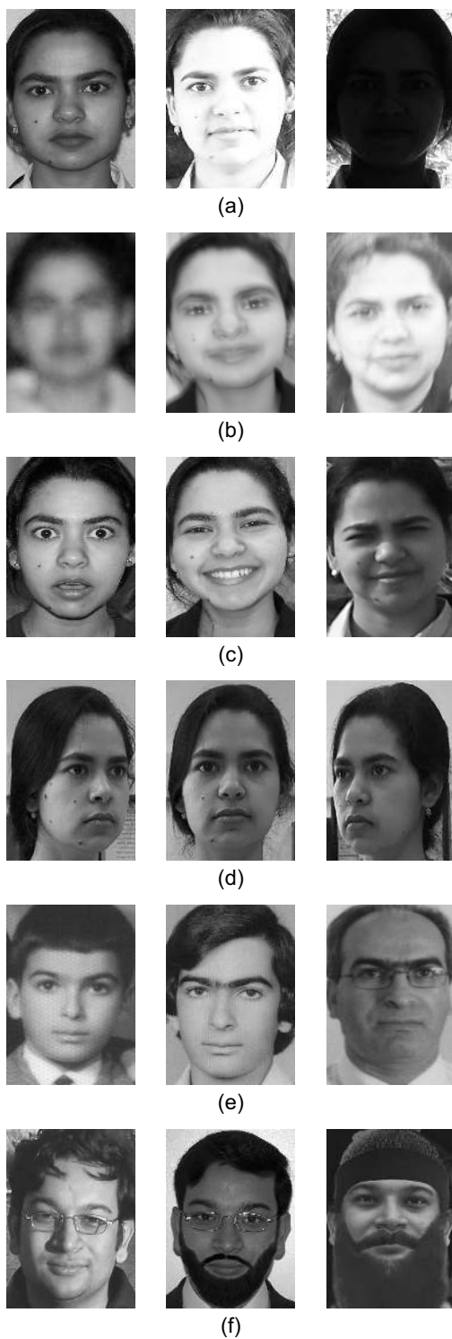
Figure 1.4: Covariates in face recognition: (a) illumination, (b) image quality, (c) expression, (d) pose, (e) aging, and (f) disguise.
