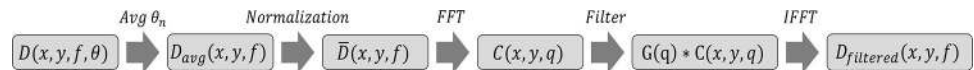
Fig 2. Signal processing flowchart. The flowchart describes the signal processing steps taken during the cepstrum analysis.
