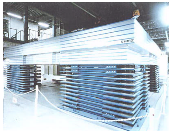
Figure 23: ORC 200 Symbol Tower and HMD unit installed inside. (taken from Yasui Architects & Engineers, Inc.)
