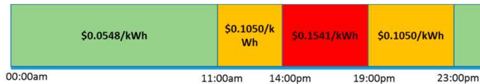
Figure 4. Time of use program (ToU) demand response (DR) signal for a summer day.
