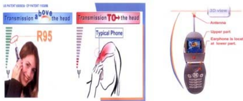
Fig4. Suggested R95 Technique Headset to Decrease Significantly the SAR in Comparison with a Typical One.
