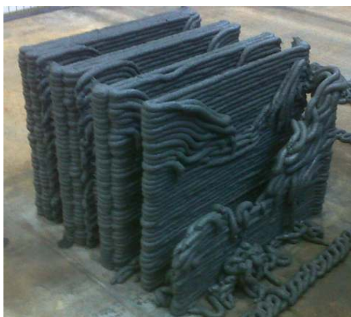
Fig. 14. The buildability of a 0.55 kPa shear strength concrete mix
