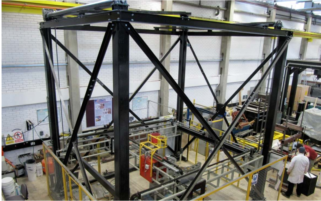
Fig. 1. Concrete printing system
