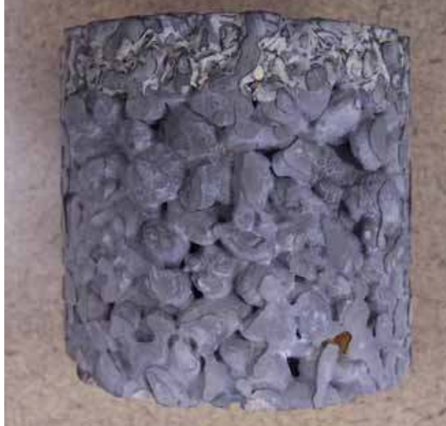
Figure A.16. Side view of PCPC, with high void continuity along sample sides
