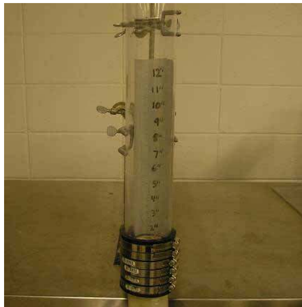
Figure 10. Permeameter used to measure the permeability of pervious concrete samples
