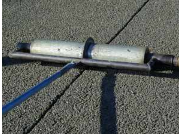
Figure 6. Roller used to make joints in pervious concrete
