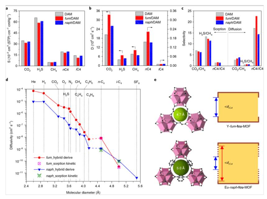
The molecular sieving properties can be finely tuned by varying the ultra-microporous structures of RE-**fcu**-MOFs using different organic linkers. The *naph* linker is, of course, longer than the *fum* linker (length of *fum*: 5.0 Å, *naph*: 6.9 Å)[29],
