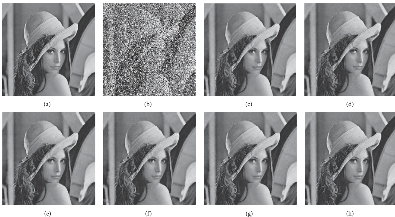
FIGURE 13: Denoising results of different methods for Lena image. (a) Noise-free image. (b) Image corrupted by mixed noise (AWGN+SPIN, \sigma=10 , p=50\% ). From (c) to (h): denoising results of Cai, AMF+LRA, AMF+LRR, WLRA, WLRR, and the proposed algorithm.
