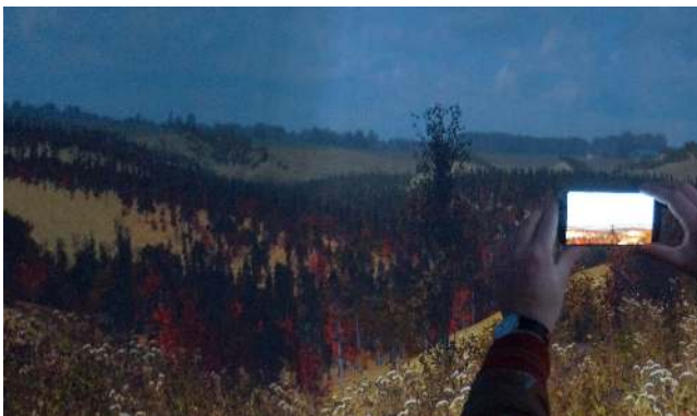
Figure 2: Mixed reality simulation using a mobile device in our display environment. The simulated real-world is shown as a backdrop and the augmenting device is shown with a rendered view that was streamed wirelessly from the simulator server.
