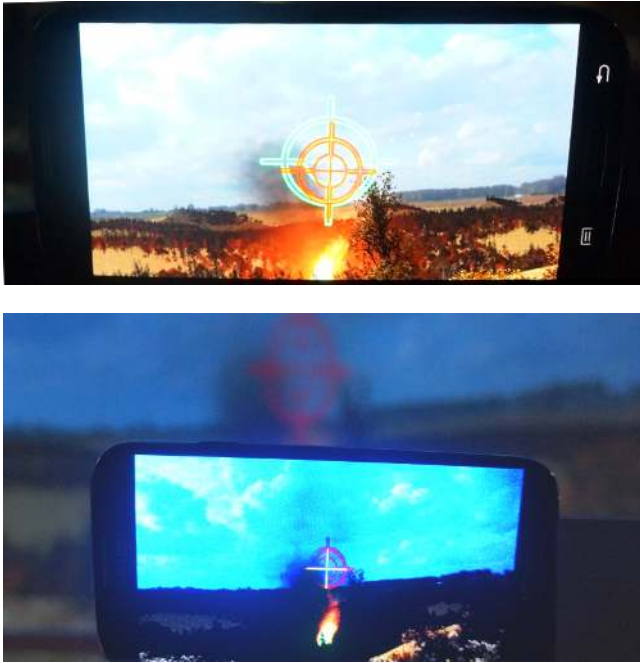
Figure 7: Top image: alignment of the augmenting device crosshair (green), with the real-world display crosshair (red). Bottom image: alignment of the back-facing camera crosshair (green), with the real-world display crosshair (red). The real-world display crosshair can also be seen in the background of the bottom image.
