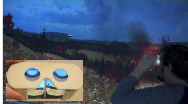
Figure 5: Use of a smart phone as a stereo binocular display, using a VR2GO mobile viewer
