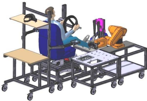
Fig. 2. The virtual representation of our seating buck. ( Color Plate 9 )
