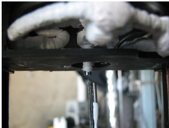
Figure 4. Thermocouple and pressure transducer probes near the exit of the coaxial injector.
