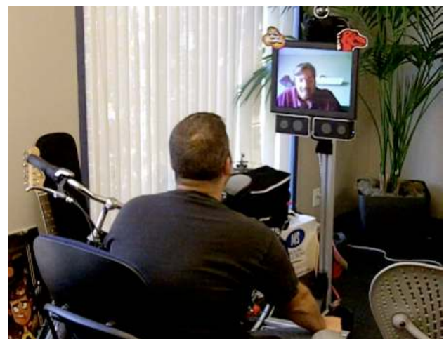
Figure 1. Remote pilot (in Boston, MA) talking with a local colleague (in Mountain View, CA) via an MRP system
