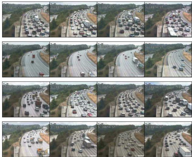
Figure 2. Example of clustering traffic video into four classes, corresponding to (top to bottom) stopped traffic, light traffic, slow traffic, and medium traffic. Four typical sequences are shown for each of the four clusters.
