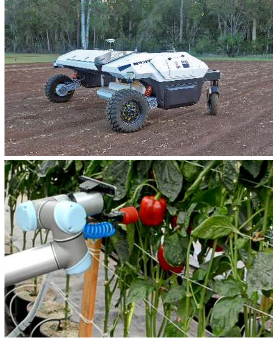
Fig. 1. Top is an image of AgBot II which performs weed management and bottom is Harvey a robotic sweet pepper harvester.
