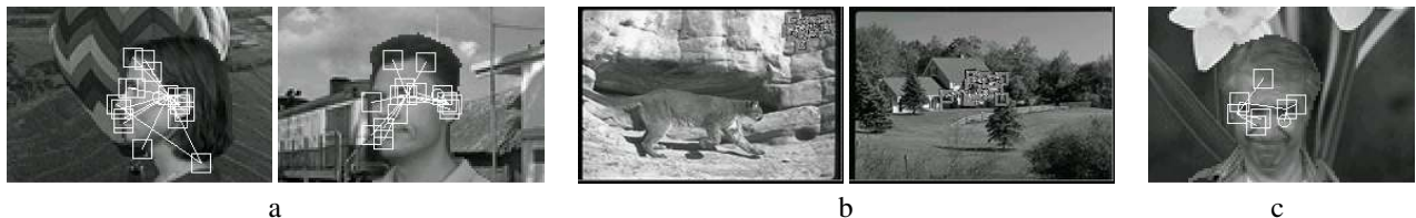
Figure 6: Examples of the view-invariant face detector applied to faces and backgrounds. (a) examples of face assemblies detected correctly. The squares show the features in the assembly, the circle corresponds to the root node of the mixture of trees, and the edges show the edges of the mixture component corresponding to the assembly. (b) False detections in background images. (c) An example of a missed detection. Even though a feature assembly is found corresponding to a face, its posterior is too low to declare a face detection.
